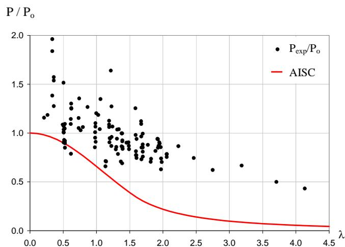
Figure 3. Experimental vs. AISC column curve for SRCs
