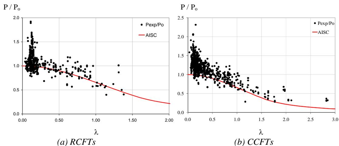
Figure 2. Experimental vs. analytical column curve for CFTs
